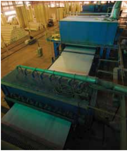
Producing spunbond roofing membrane reinforcement and geotextiles at Spuntex factory
