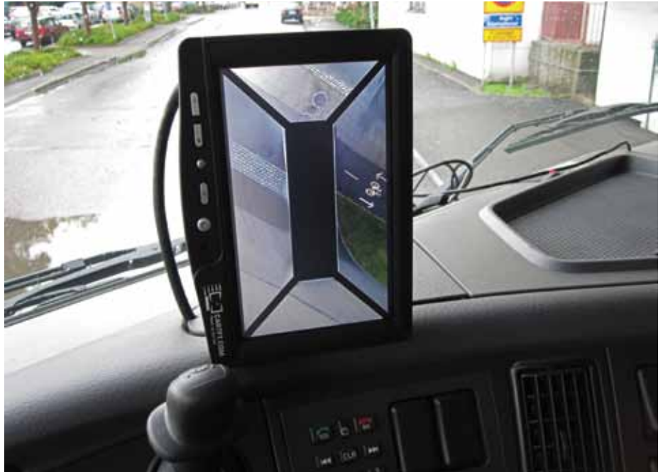
Fitting laser scanners and ultrasonic sensors that monitor the area on the truck's passenger side in order to reduce accidents
