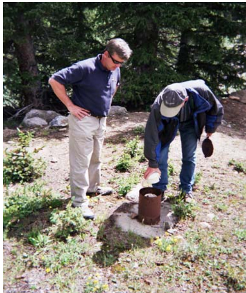
Figure 4. Observation well downstream of dam.
