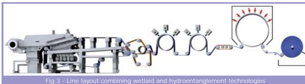
Fig.3 - Line layout combining wetlaid and hydroentanglement technologies
