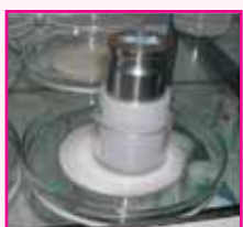
Source: EDANA Apparatus For measuring absorbency, under pressure, of PA superabsorbent powders
