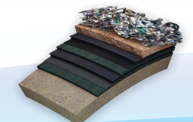
Cross-Section of a bottom liner in a landfill (top) and liquid containment (bottom) using GCL technology.
