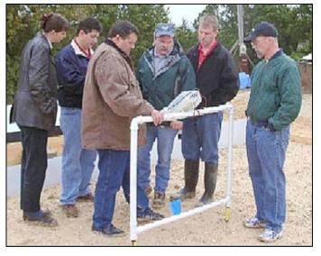
application technology with the use of electrical current to detect holes/leaks in lining systems.
