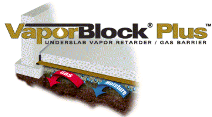
Radon and vapor barrier and concrete liners
