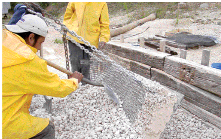
Photo 2. Tilting up of the underlying steel plates facilitates exhumation of samples without further damage.
