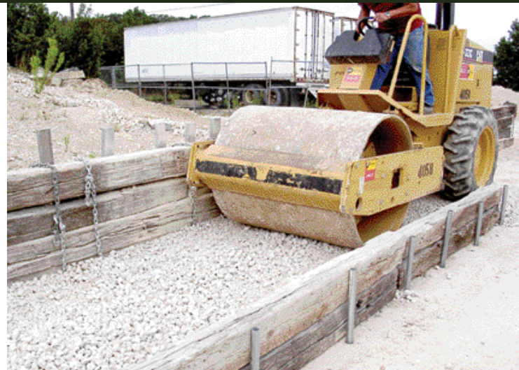
Photo 1. Geosynthetic samples are installed and exposed to field-scale placement and compaction stresses.
