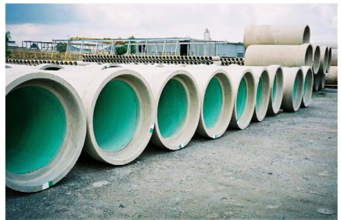
The complete AKS lined pipes ready for transport to site.
