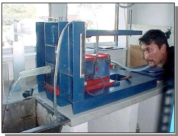
Geosynthetic Laboratory’s old transmissivity test rig
