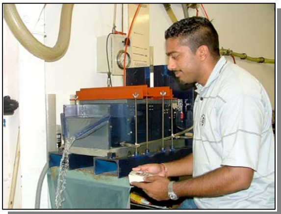
Geosynthetic Laboratory’s new transmissivity test rig
