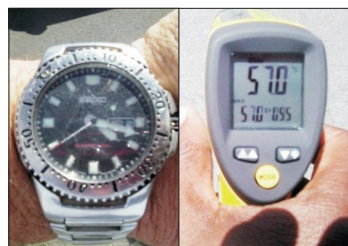
Road surface temperature of 57 degrees Celcius at 16:15 in the afternoon whilst installing the Fibertex geotextile, Route B1 Namibia - 2012
