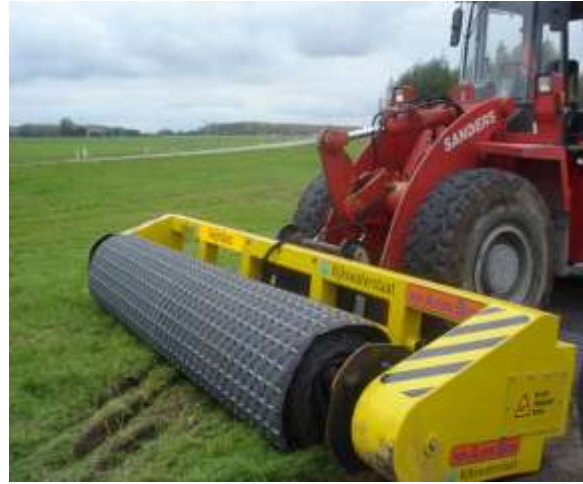
Figure 10. Light and heavy portable access roads (compl. Robusta Mats™).
