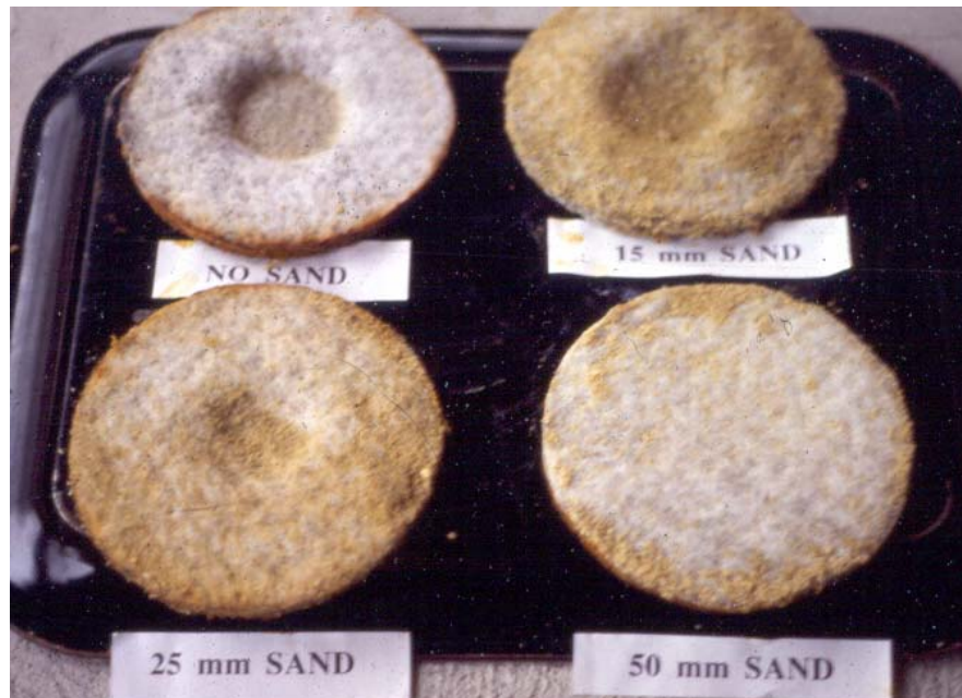
Figure 2. Results of Tests on Thinning of Bentonite beneath a Loaded Area for a Geotextile-Encased GCL (Koerner and Narejo, 1995)
