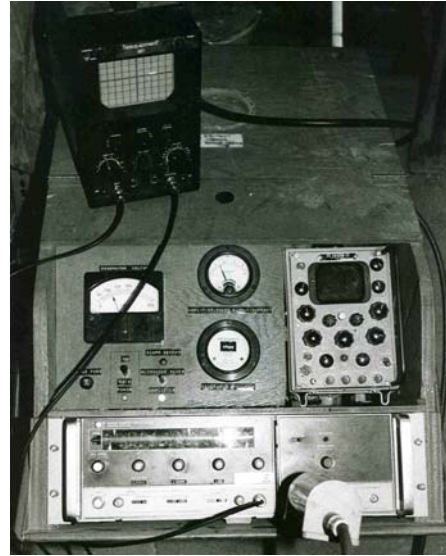
Figure 2 – Continuous wave microwave unit designed and manufactured in the Drexel University nondestructive evaluation techniques research program by Koerner and Lord (c1980).
