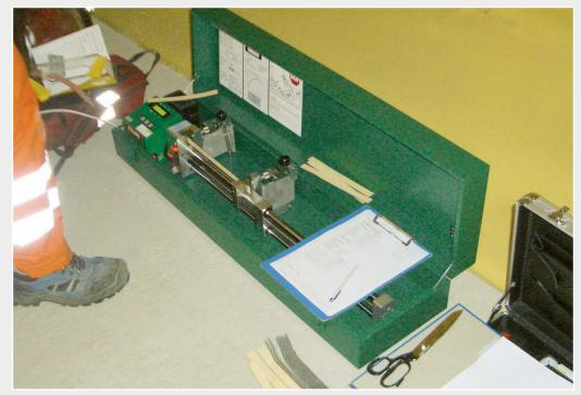
Peel tests are conducted in the laboratory, but also on site with the EXAMO test device from Leister.
