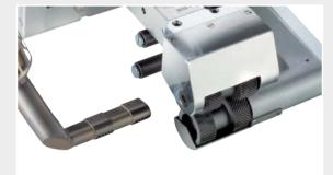
the weld quality. To guarantee the greatest possible safety here, a test channel is installed for each overlap weld. This is realised with the pressure roller on the TWINNY S which was specially designed for this purpose. This ensures two parallel weld seams of 0.6 inch each. The resulting test channel between these seams is 0.8 inch wide. The watertightness can be reliably monitored via compressed air using this channel.
