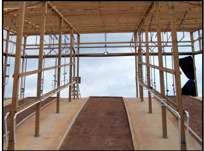
DDRF covered slope erosion test facility
